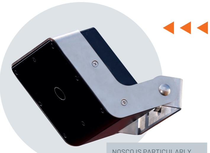
The NOSCO.hybridcamera fuses the data of two sensors (camera and radar), which are located in the entry and exit areas or on the ramps of parking garages. The NOSCO.engine signal processing unit evaluates the data from the NOSCO.hybridcamera and transmits it to the LOBO.control software, which controls the displays in the parking garage.
